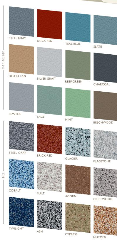
All samples shown are coated. Stonhard coatings include high solids and solvent-based epoxies and urethanes. All coatings are available in the colors shown here in addition to Clear, Black and OSHA Safety Yellow. Urethane coatings are also available in White.
